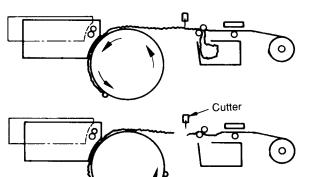
The Drum rotates intermittently to load the master material while the master making is continued.
